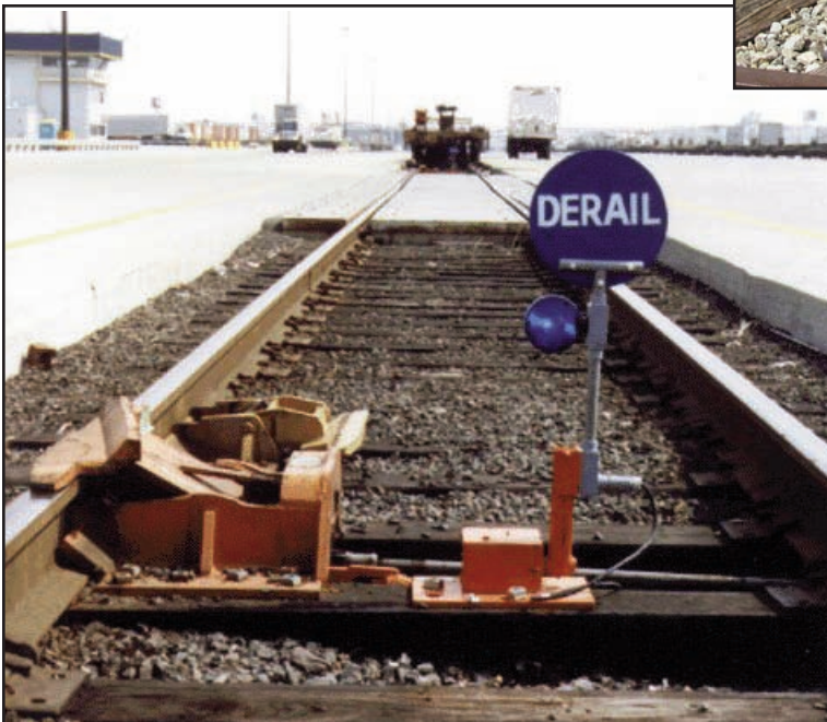
Automatic Mechanical Blue Flag which activates when a derailer is activated.
