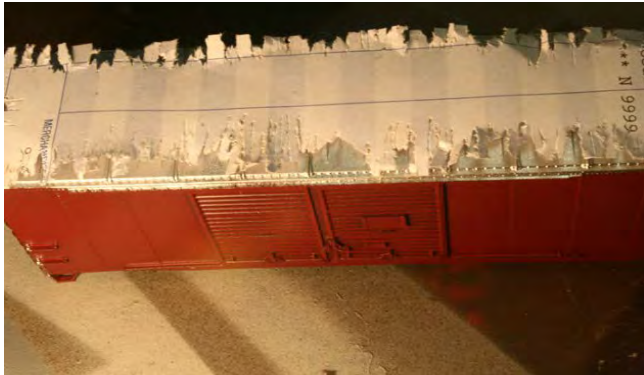
Above: The paper mask applied to the roof of a boxcar prior to painting Right: The painted car demonstrating the nice overspary detail Below: painted roof and the paper mask that created the effect
