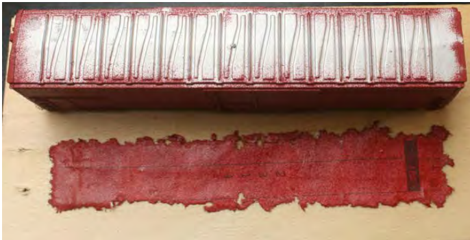
Above: The paper mask applied to the roof of a boxcar prior to painting Right: The painted car demonstrating the nice overspary detail Below: painted roof and the paper mask that created the effect
