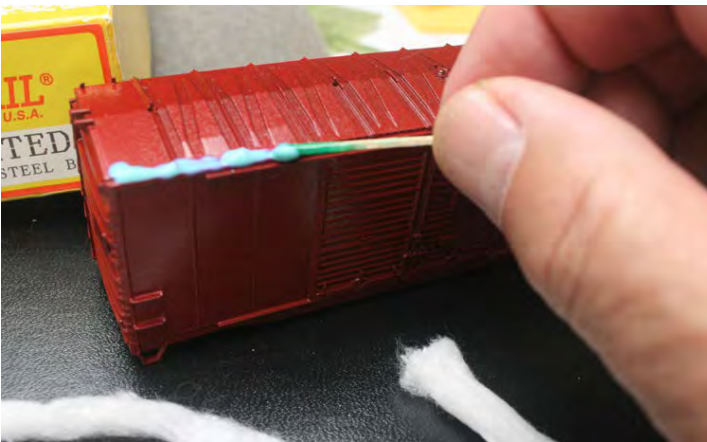
Above: Apply the cotton strips to the EZ Mask along the edges. The idea is to get a feathered effect when the paint is sprayed. Do not forget to mask the entire car
